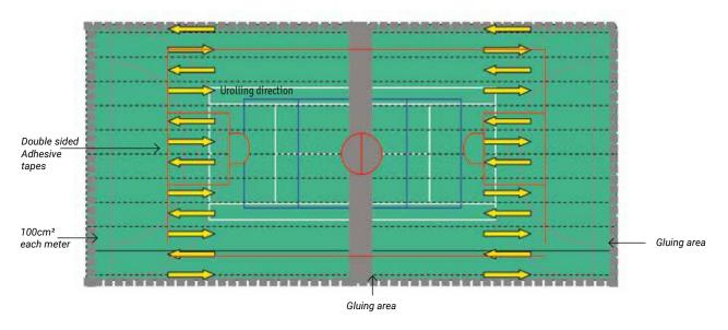
We recommend a dual-component epoxy glue, GreenLay Glue, reference Component A 1551057 Component B 1551058 – quantity to be applied, with a thin set of teeth spatula, between 300 and 350 gr per sqm. For a good installation you must carefully follow the manufacturer recommendations in particular, the waiting time before applying the covering. Then the surface with a roller to eliminate any bubbles that might remain between the sub-floor and the covering.
