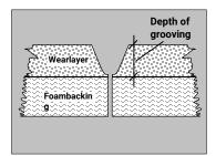
The grooving depth of seams must never be deeper than 2/3 of the thickness of the wearlayer.
