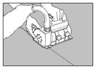
The joints are chamfered or grooved to about 2/3 of the thickness using a hand grooving tool or machine prior to welding. Never reach the foam backing when existing.
