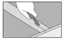
Fix a special masking tape, centered over the cut seam, then cut the masking tape with a rolling knife within the seam.
