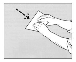
Press the sheet firmly using a piece of board with rounded edge or equivalent tool. Work from top down and from the middle to the sides of the sheet.
