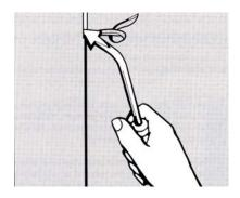
All seams are grooved using hand groover. Groove until 2/3 of the thickness.
