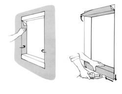
For best result, extra heating and pressing is necessary to secure a good bonding at overlapping areas.
