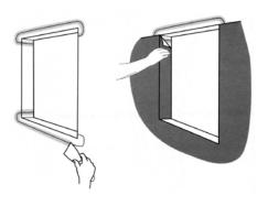
Alternative 2: At window-recesses the wall covering is rolled out over the window area and is then folded into the reveals. Loose pieces are inserted at the bottom recess, and at the top recess where necessary. The loose pieces are joined to the wall covering with welded seams.
